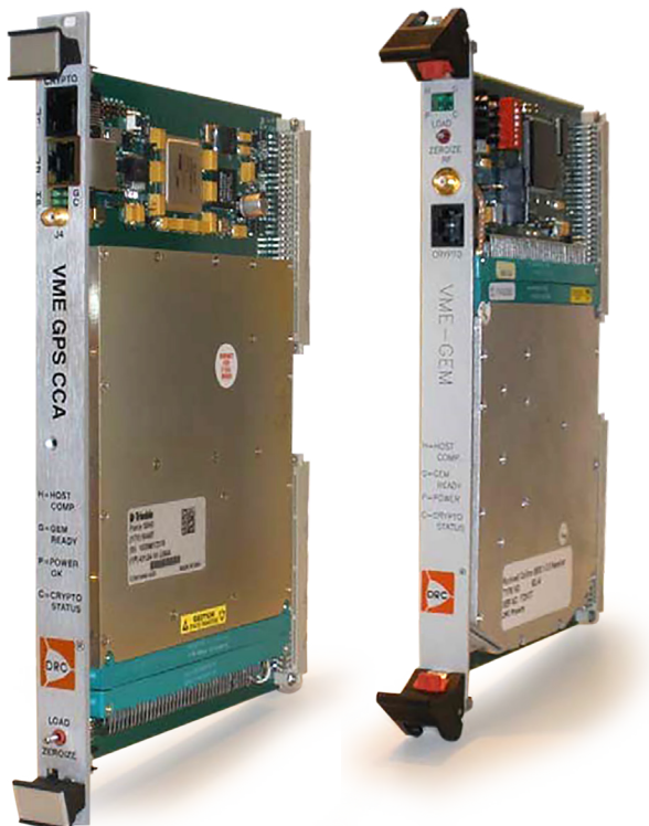
Figure 1: Comparison of VME-GPS CCA P/N 510000 (left) shown next to VME-GEM CCA P/N 500400 (right)
