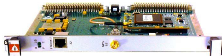
VME Host Adapter for Military-Qualified 12/24-Satellite Channel GPS Receiver with Selective Availability Anti-Spoofing Module (SAASM)
