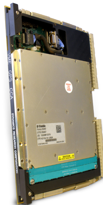
VME Host Adapter for Military-Qualified 12/24-Satellite Channel GPS Receiver with Selective Availability Anti-Spoofing Module (SAASM)
